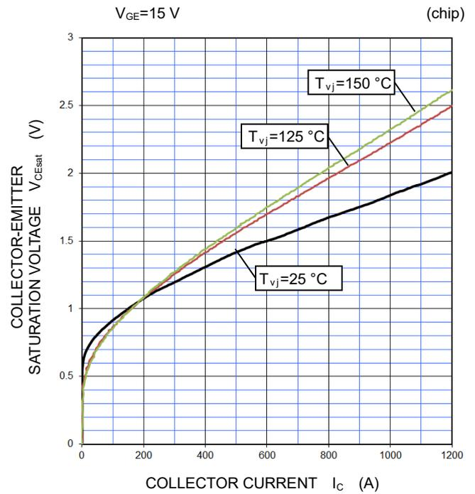
**COLLECTOR-EMITTER VOLTAGE CHARACTERISTICS (TYPICAL)**
