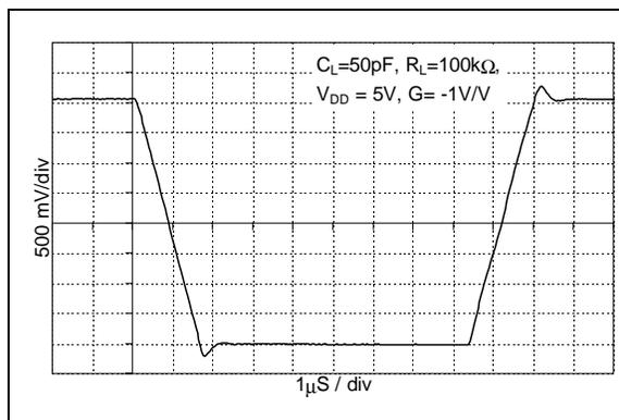
**FIGURE 2-28:** Large Signal Inverting Signal Pulse Response
