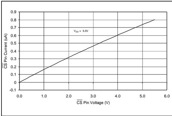
**FIGURE 2-31:** Input  $\overline{CS}$  Current vs.  $\overline{CS}$  Voltage
