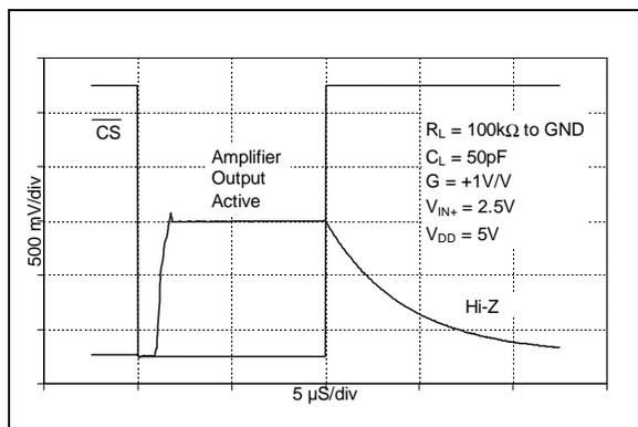
**FIGURE 2-27:** Chip Select to Amplifier Output Response Time
