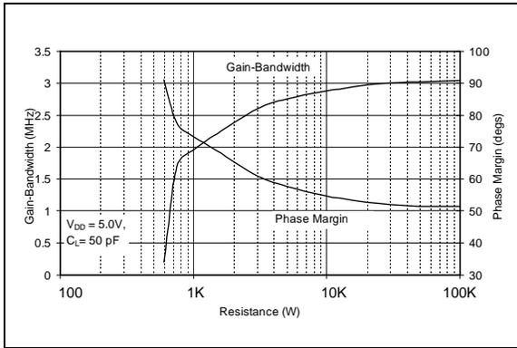
**FIGURE 2-19:** Gain Bandwidth, Phase Margin vs. Load Resistance
