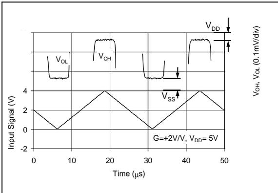
**FIGURE 3-1:** Low Level and High Level Output Swing
