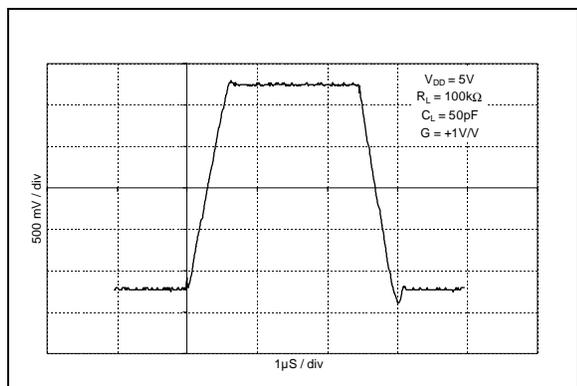
**FIGURE 2-25:** Large Signal Non-Inverting Signal Pulse Response
