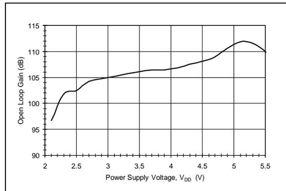
**FIGURE 2-18:** DC Open Loop Gain vs. Power Supply
