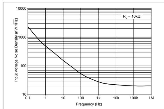
**FIGURE 2-6:** Input Voltage Noise Density vs. Frequency
