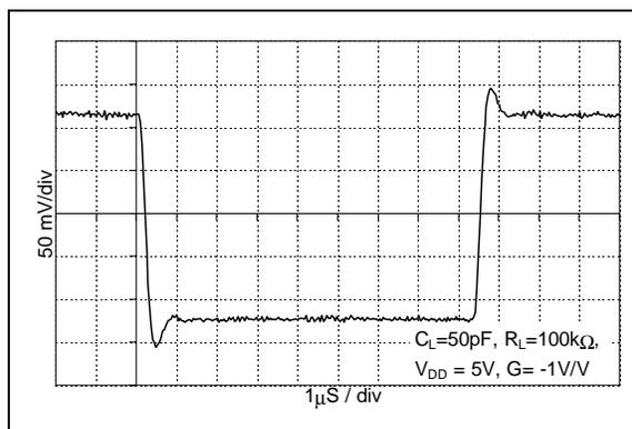
**FIGURE 2-29:** Small Signal Inverting Signal Pulse Response
