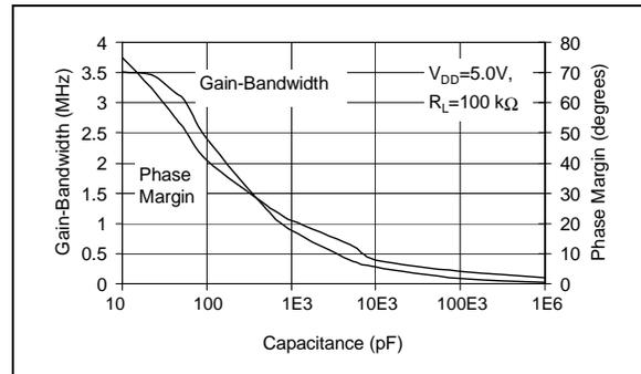
**FIGURE 3-4:** Gain Bandwidth, Phase Margin vs. Capacitive Load
