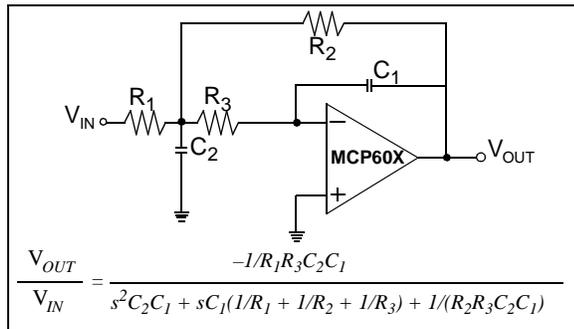
**FIGURE 3-11:** 2nd Order Low Pass Multiple-Feedback Filter
