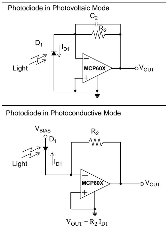
**FIGURE 3-14:** Photo Sensing Circuits Using the MCP60X Amplifier
