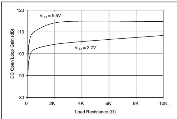
**FIGURE 2-15:** DC Open Loop Gain vs. Output Load
