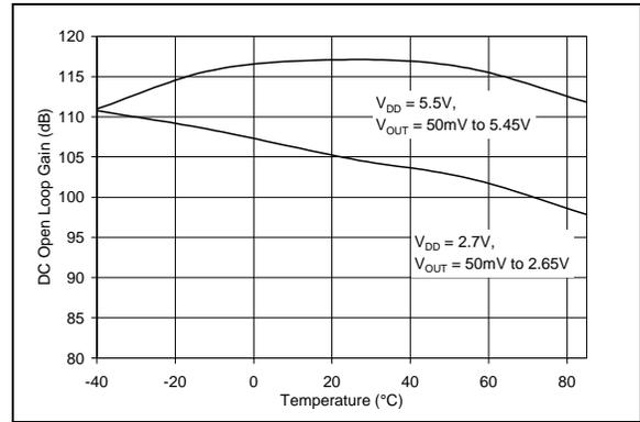
**FIGURE 2-22:** DC Open Loop Gain vs. Temperature
