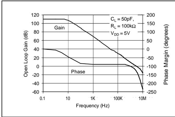
**FIGURE 2-1:** Open Loop Gain, Phase Margin vs. Frequency
