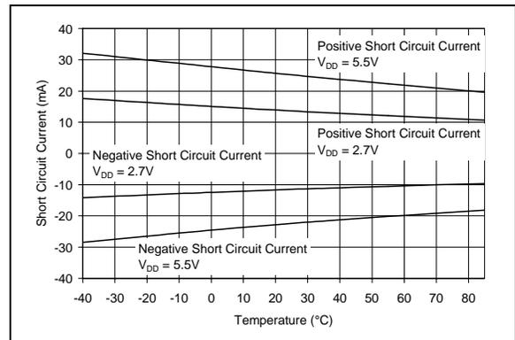
**FIGURE 2-24:** Output Short Circuit Current vs. Temperature
