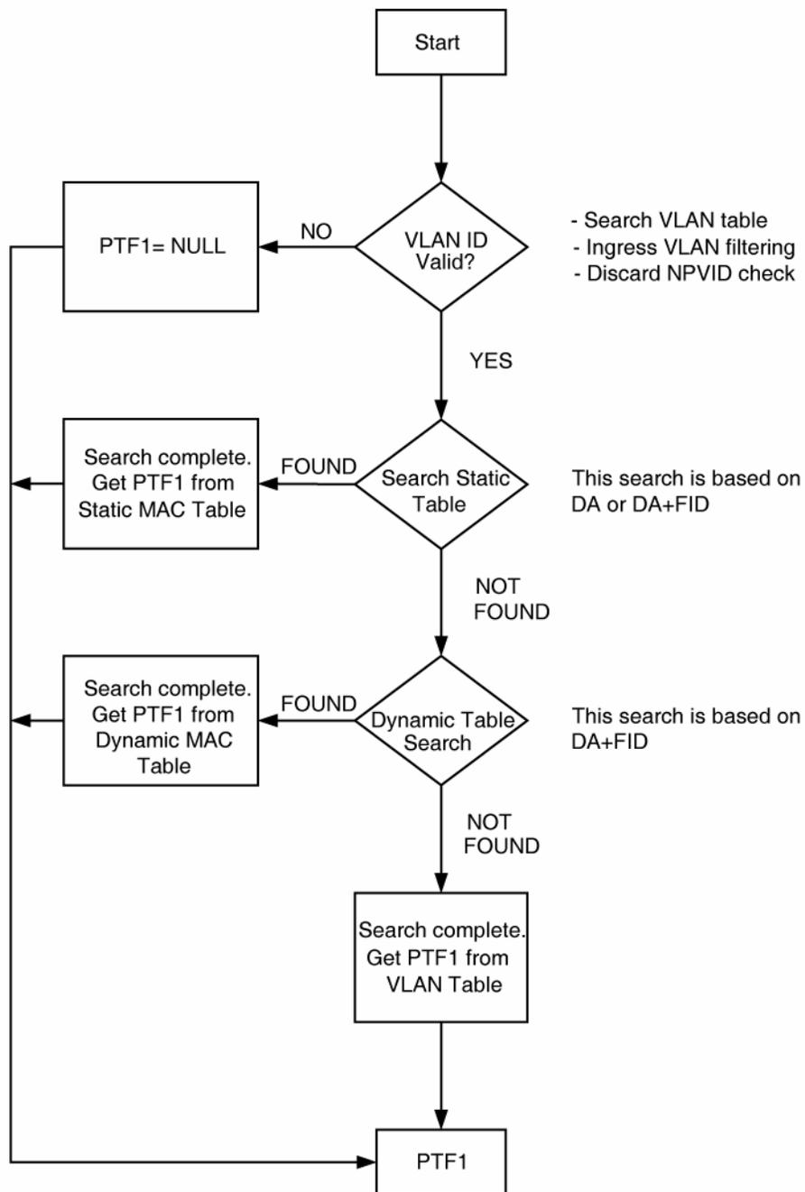
Figure 4. Destination Address Lookup Flow Chart, Stage 1
