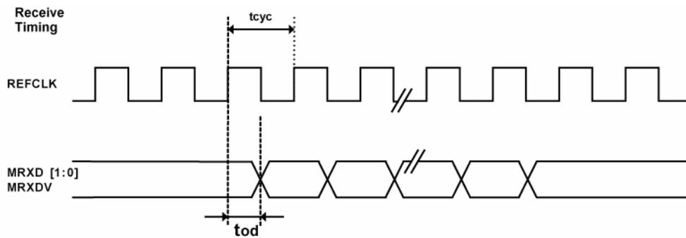
**Figure 23. RMII Timing – Data Transmitted to RMII**
