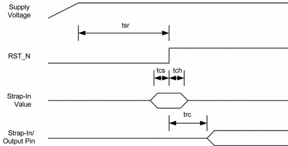
**Figure 31. Reset Timing**
