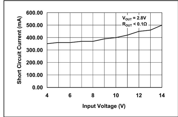
**FIGURE 2-18:** Short Circuit Current vs. Input Voltage.
