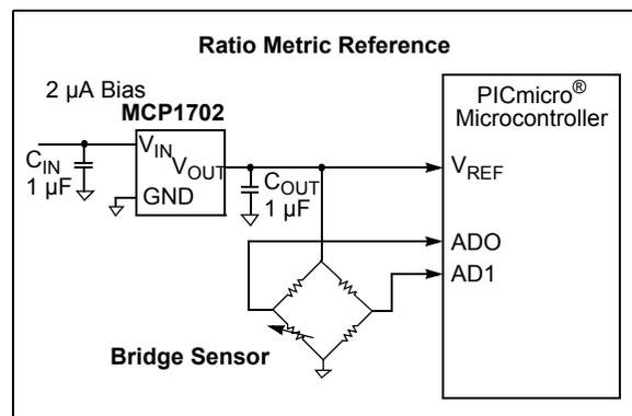
**FIGURE 6-2:** Using the MCP1702 as a voltage reference.
