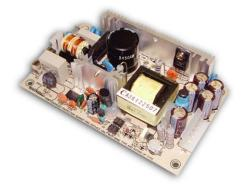
5. Mounting holes M1 and M2 should be grounded for EMI purposes.
