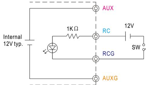
Example 3.2(B): Using internal 12V auxiliary output
