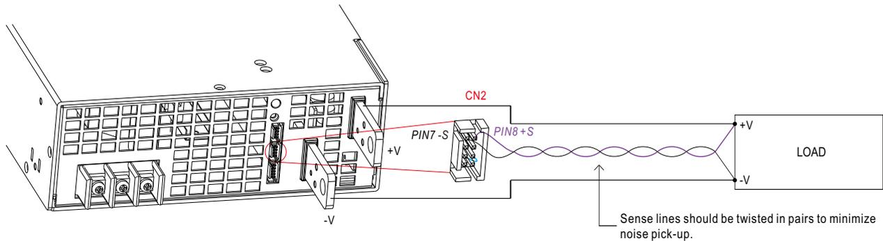
※ Caution: The power supply, by factory default (also the assumption for other sections), is shipped with, -S & -V on CN2, as well as +S & +V, shorted by connector. When activating the Remote Sense, the +S signal should be connected to the positive terminal of the load whereas -S signal to the negative terminal.
