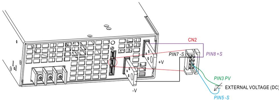
◎ Connecting an external DC source between PV & -S on CN2, and +S & +V, -S & -V also need to be connected as exhibited above.
