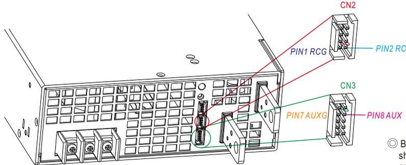
◎ By factory default, PV(PIN3) and PS(PIN4) on CN2 are shorted by connector; likewise, OLP(PIN9) and OL-SD(PIN10) on CN3 are shorted when shipped.
