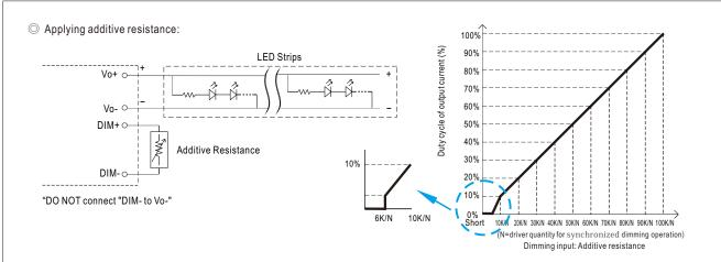
Note: 1. Min. duty cycle of output current is about 6% and the output current is not defined when 0% Iout<6%. 2. The duty cycle of output current could drop down to 0% when dimming input is about 0% or 0% or 0% or 0% or 0% duty cycle.
