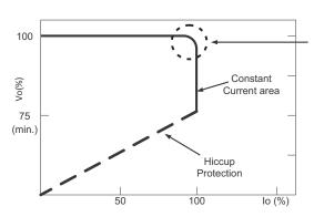
Typical LED power supply I-V curve
