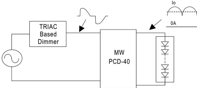
Under direct driving, the power supply will work in "constant current mode (CC)" and output voltage of the power supply will be clamped by sum of forward voltage (V<sub>F</sub>) of the LED strip.
