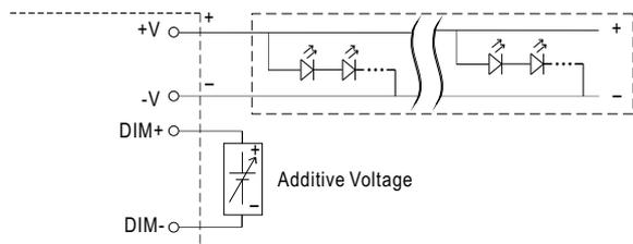
"DO NOT connect "DIM- to -V"
