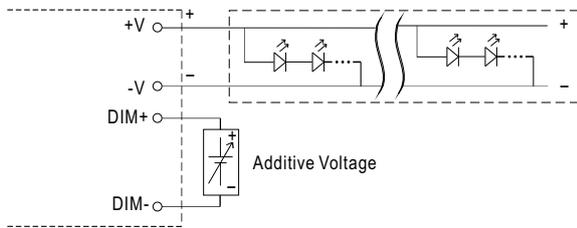
"DO NOT connect "DIM- to -V"
