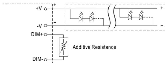
"DO NOT connect "DIM- to -V"
