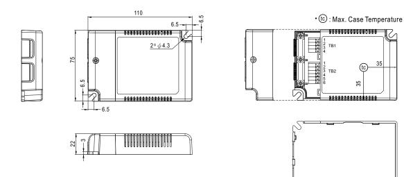
NOTE: Please use wires with a cross section of 0.75~1.5mm² for TB1 and wires with a cross section of 0.5~1.5mm² for TB2.
