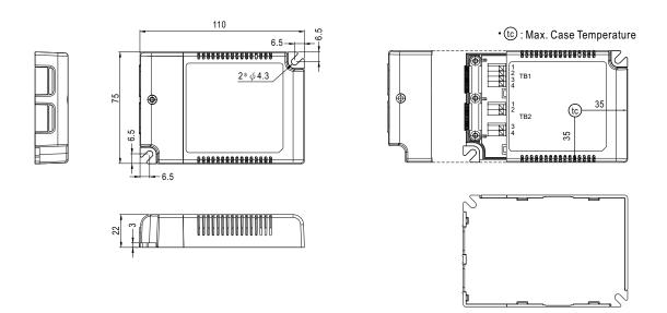
NOTE: Please use wires with a cross section of 0.75~1.5mm² for TB1 and wires with a cross section of 0.5~1.5mm² for TB2.
