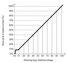
O Applying additive 10V PWM signal (frequency range 300~3KHz):
