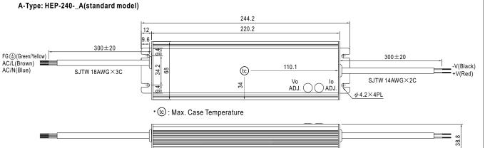
※ IP65 rated. Output voltage and constant current level can be adjusted through internal potentiometer. (Can access by removing the rubber stopper on the case.)
