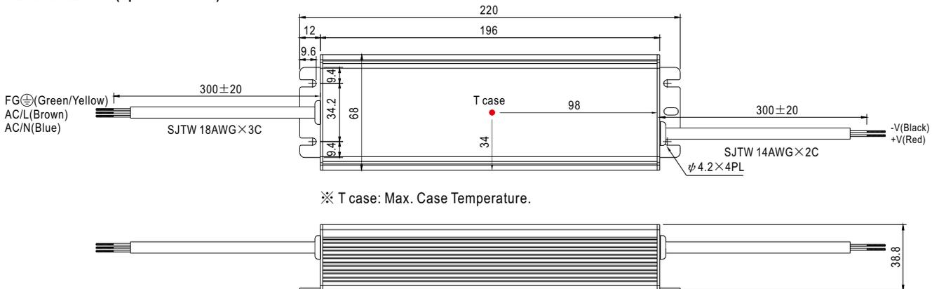
※ IP68 rated. Cable for I/O connection.
