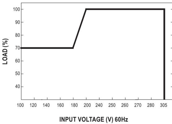
※ De-rating is needed under low input voltage.
