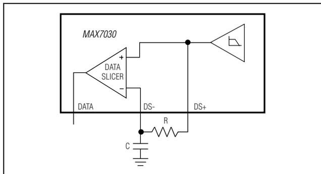
Figure 2. Generating Data-Slicer Threshold Using a Lowpass Filter
