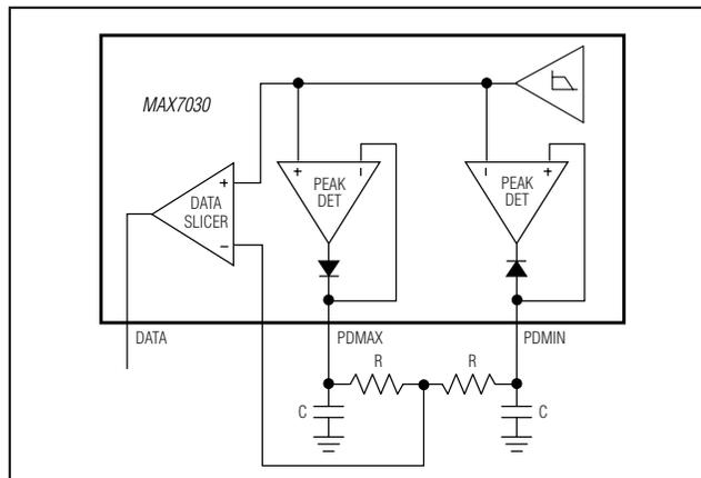
Figure 3. Generating Data-Slicer Threshold Using the Peak Detectors
