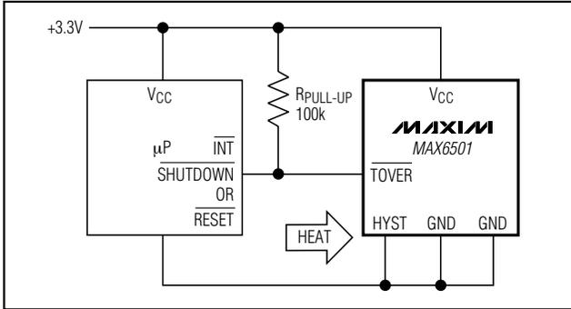
Figure 2. Microprocessor Alarm/Reset
