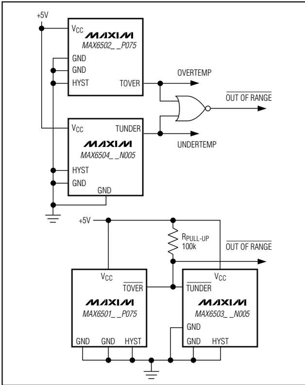
Figure 4. Temperature-Window Alarms
