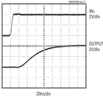
**INPUT VOLTAGE vs. OUTPUT VOLTAGE**
