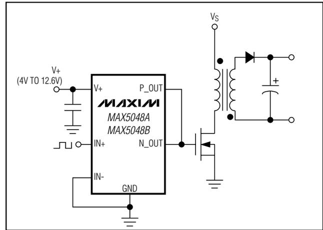
Figure 3. Noninverting Application
