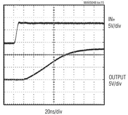
**INPUT VOLTAGE vs. OUTPUT VOLTAGE**
