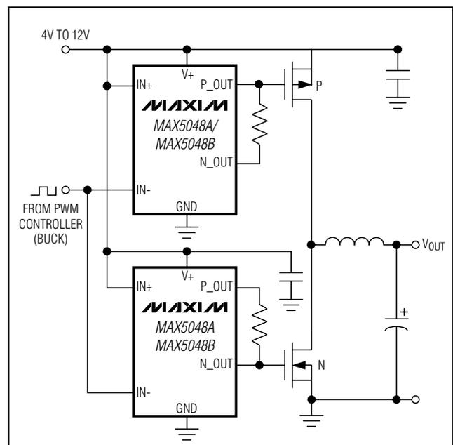
Figure 5. MAX5048A/MAX5048B in High-Power Synchronous Buck Converter
