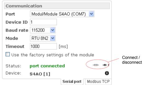
Figure 14: Establishing connection to S4AO module
