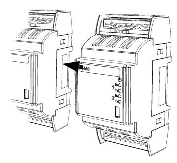
Figure 6: lateral bus connection
