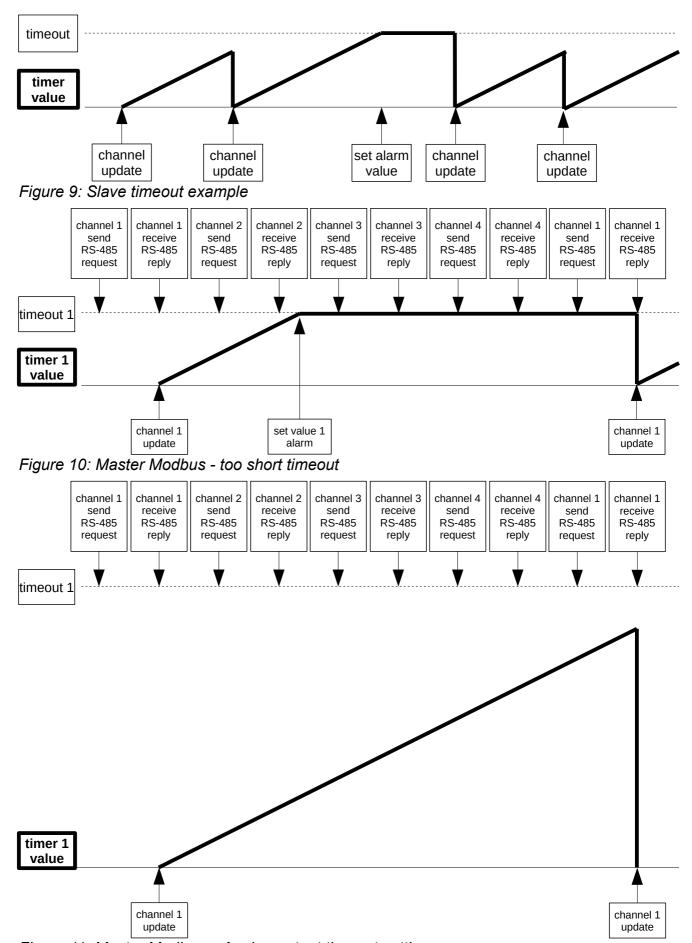
Figure 11: Master Modbus - Analog output timeout setting
