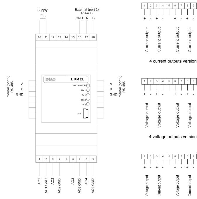
Figure 3: Electrical connections of the S4AO module.
