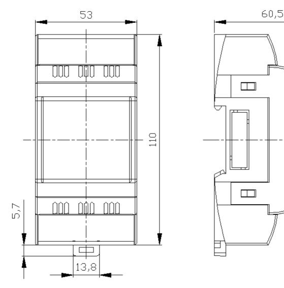
Figure 2: Module dimensions
