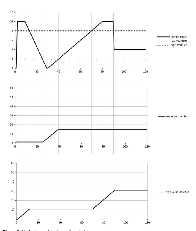
Figure 7: High / low value timers thresholds
