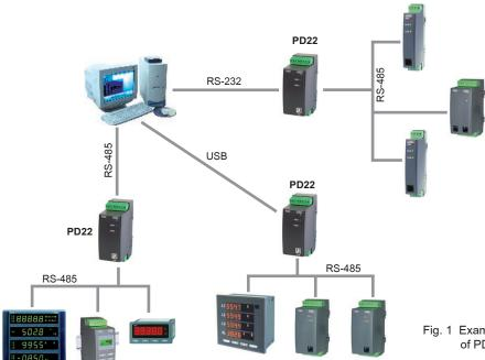
Fig. 1 Examplary network topology with the application of PD22 data loggers
