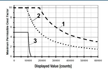
Additional error caused by signal's crest factor: 1 < CF < 3: 1% R+ 30D 3 < CF < 10: 3% R
