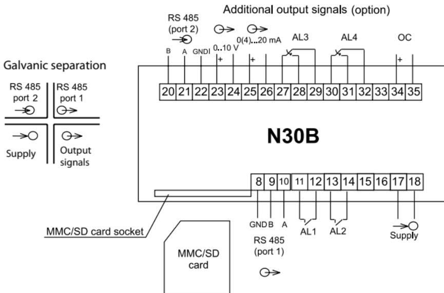
**Fig. 4. Description of signals on connection strips.**
