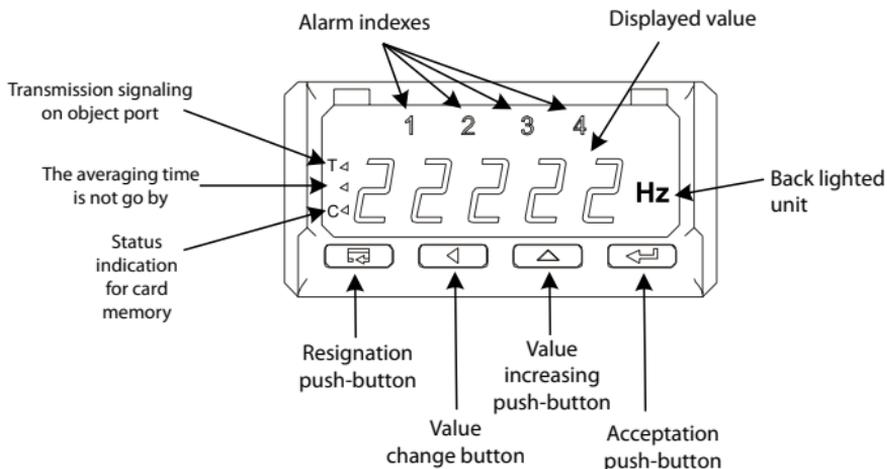
**Fig. 5. Description of the recorder frontal plate.**
