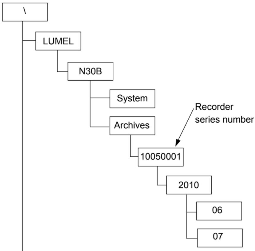
**Fig. 13 Catalogue structure in the memory card.**
