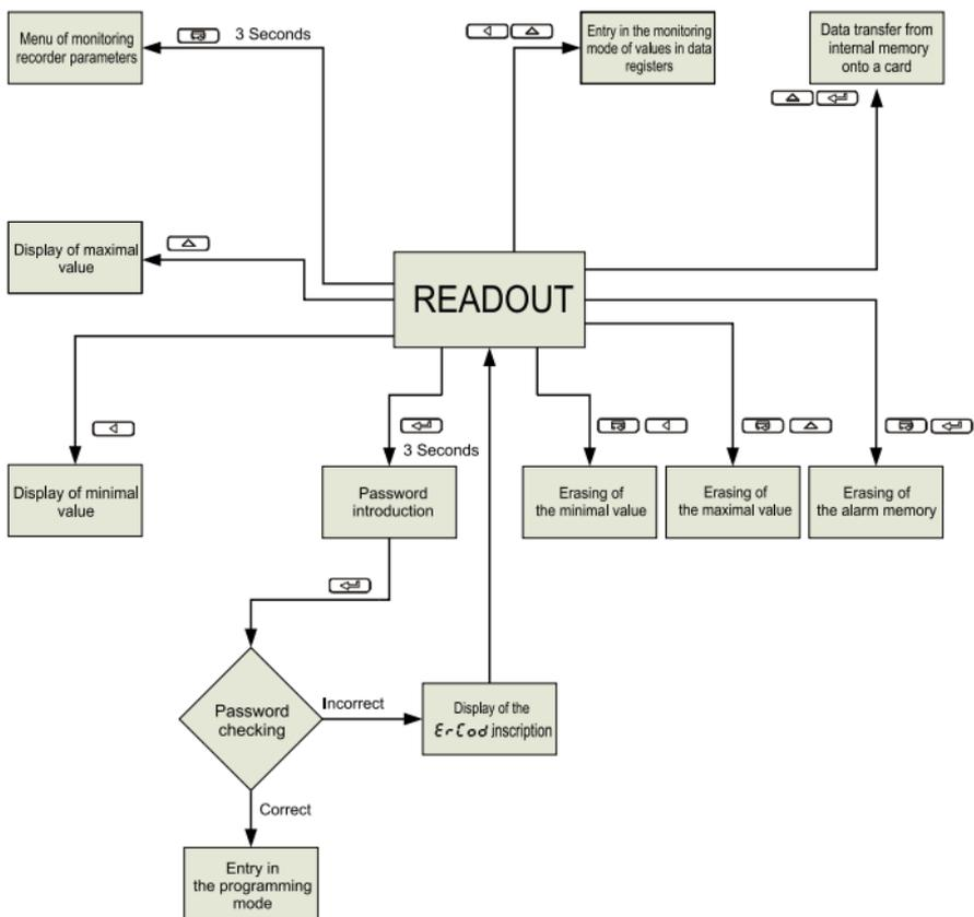
**Fig. 6. Service algorithm of the N30B recorder.**
