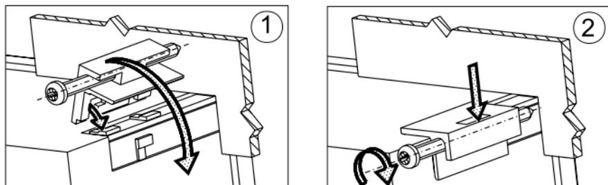
**Fig. 2. Recorder fixing.**
