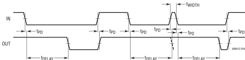
Figure 4. Falling-Edge Delayed Timing Diagram (LTC6994-1, POL = 1)
