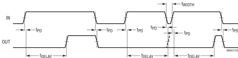
Figure 3. Rising-Edge Delayed Timing Diagram (LTC6994-1, POL = 0)
