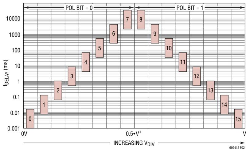
**Figure 2. Delay Range and POL Bit vs DIVCODE**
