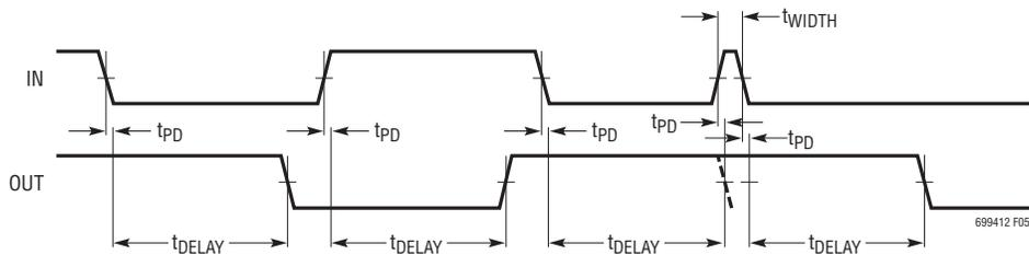
Figure 5. Both Edges Delayed Timing Diagram (LTC6994-2,  $POL = 0$ )
