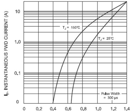
Fig. 2 Typical Fwd Characteristics
