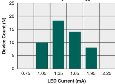
**Typical I<sub>F</sub> for Switch Dropout**
