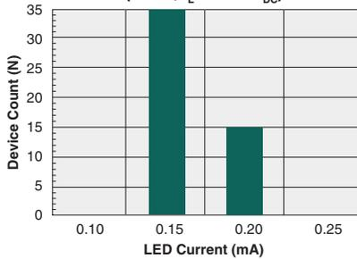
Typical  $I_F$  for Switch Dropout
