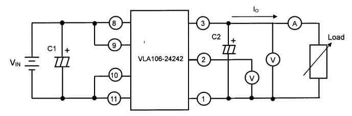
C1 : 100µF 50V (low impedance) C2 : 47µF 50V (low impedance)
