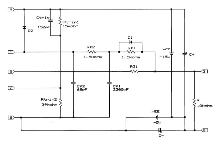
Rf1, Rf2, Cf1, Cf2, D1, D2: Parts for Noise filter circuits Rtrip1, Rtrip2: Parts for reduction of inner circuit's impedance
