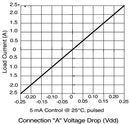
Figure 3. Linearity Characteristics
