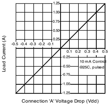
Figure 3. Linearity Characteristics
