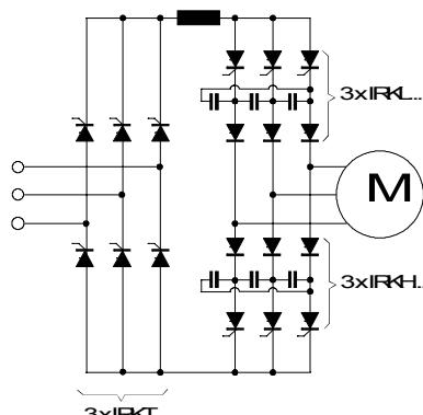
Current Source Inverter using 9 MAGN-A-paks
