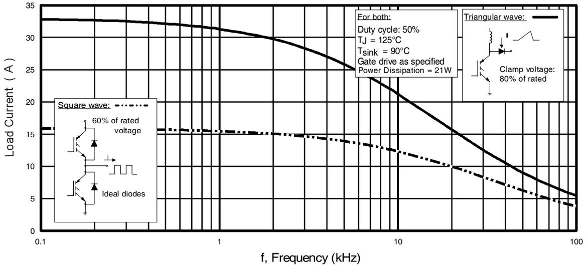
**Fig. 1 - Typical Load Current vs. Frequency**
