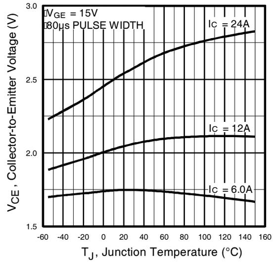
**Fig. 5 - Collector-to-Emitter Voltage vs. Junction Temperature**
