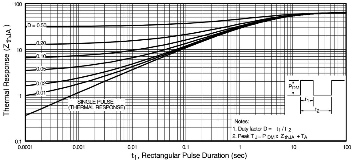
**Fig 23.** Maximum Effective Transient Thermal Impedance, Junction-to-Ambient
