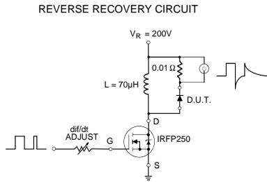
**Fig. 9** - Reverse Recovery Parameter Test Circuit
