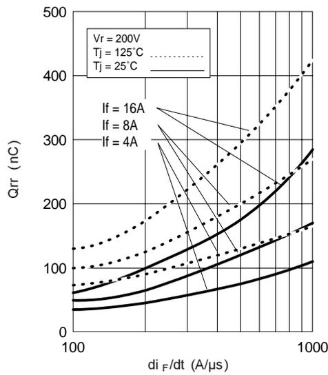
Fig. 7 - Typical Stored Charge vs.  $di_F/dt$
