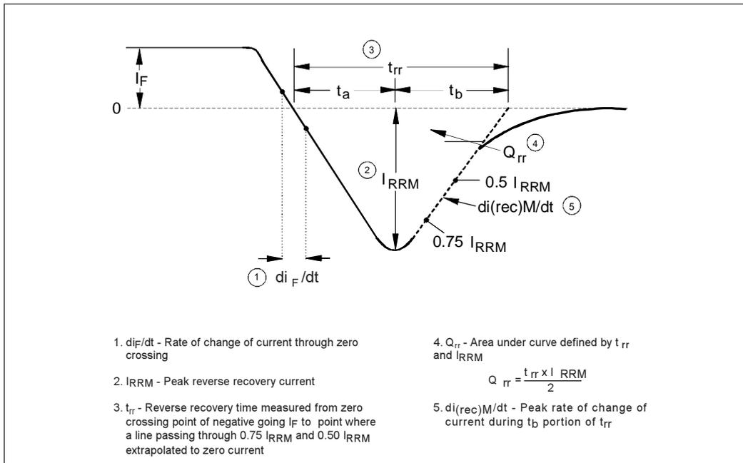
Fig. 10 - Reverse Recovery Waveform and Definitions
