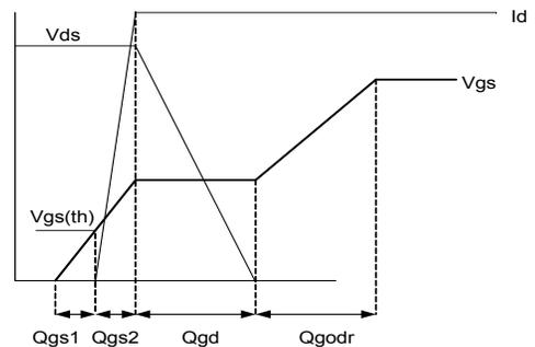
**Fig 26b. Gate Charge Waveform**
