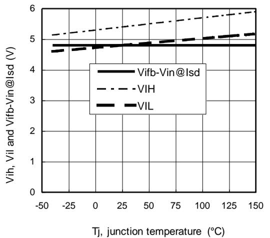
**Figure 9 – V<sub>ih</sub>, V<sub>il</sub> and V<sub>ifb-Vin@Isd</sub> (V) Vs T<sub>J</sub> (°C)**
