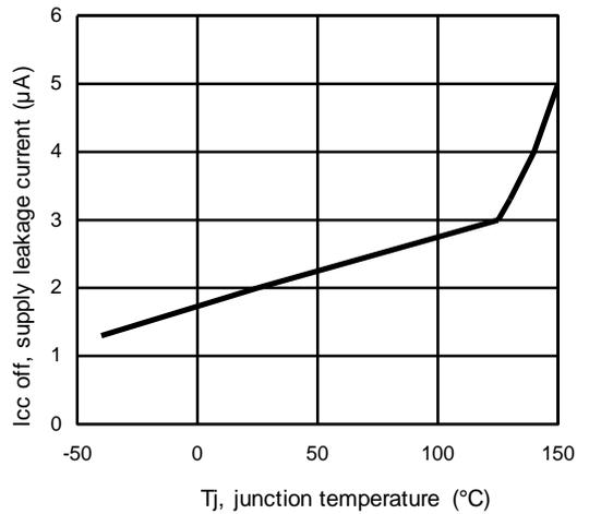
**Figure 7 – I<sub>cc off</sub> (µA) Vs T<sub>J</sub> (°C)**
