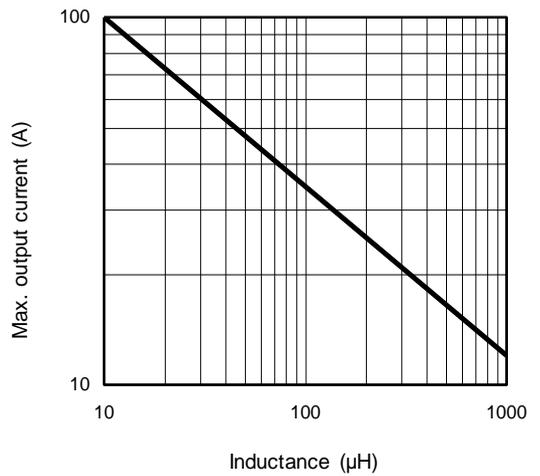
**Figure 13 – Max. iout (A) Vs inductance (μH)**
