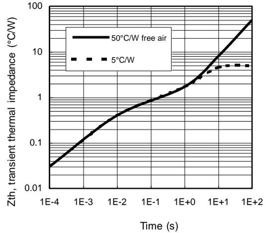
**Figure 15 – Transient thermal impedance (°C/W) Vs time (s)**
