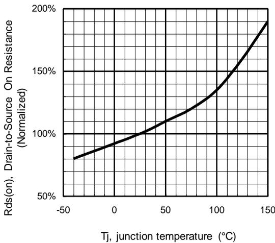
**Figure 8 - Normalized R<sub>ds(on)</sub> (%) Vs T<sub>J</sub> (°C)**
