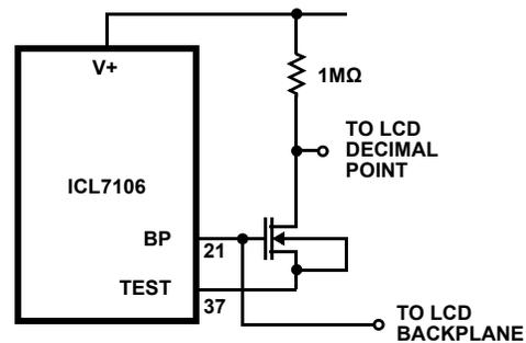
FIGURE 5. SIMPLE INVERTER FOR FIXED DECIMAL POINT
