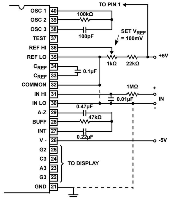
Values shown are for 200mV full scale, 3 readings/sec. IN LO may be tied to either COMMON for inputs floating with respect to supplies, or GND for single ended inputs. (See discussion in ["Analog COMMON" on page 7.](#))
