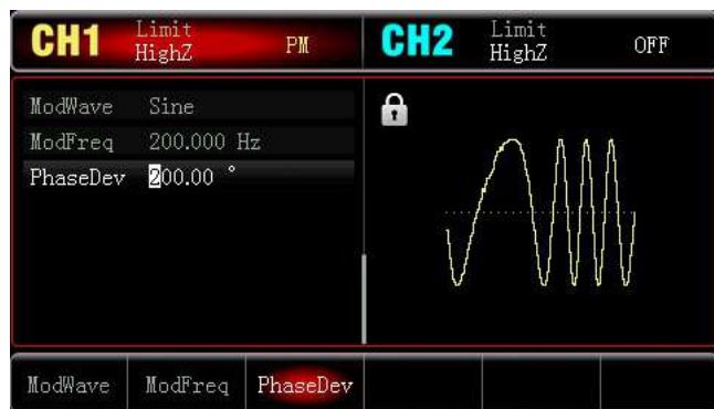
The PM modulation waveform in oscilloscope is shown below:
