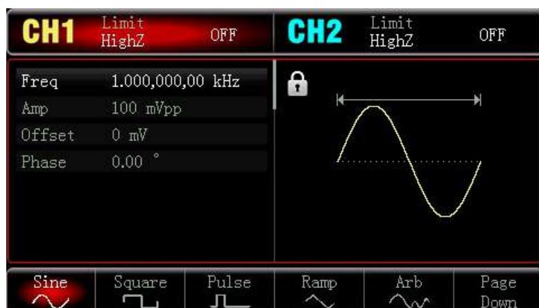
Press **Amp** to set amplitude, enter 1 by numeric keypad, and select parameter unit **Vpp**.
