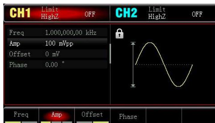
Press **Freq** to set frequency, enter 2 by numeric keypad, and select parameter unit **kHz**.
