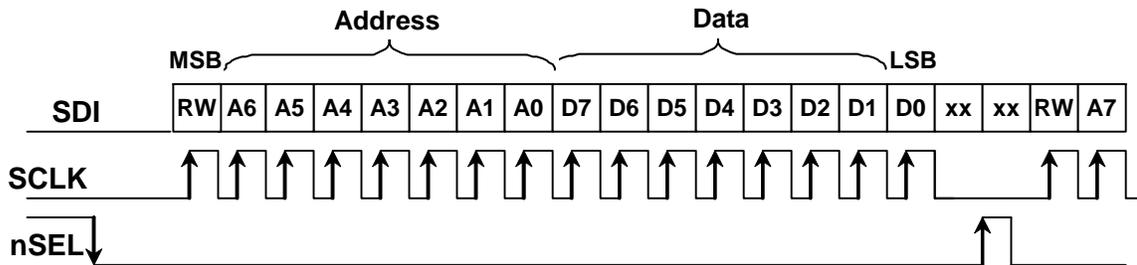
Figure 2. SPI Timing
