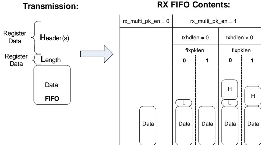
Figure 13. Multiple Packets in RX Packet Handler
