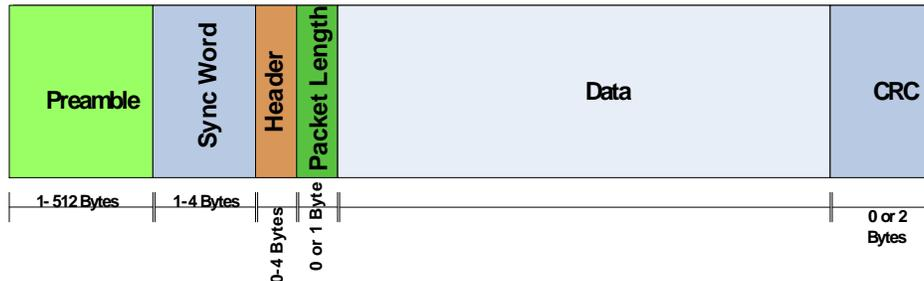
**Figure 11. Packet Structure**
