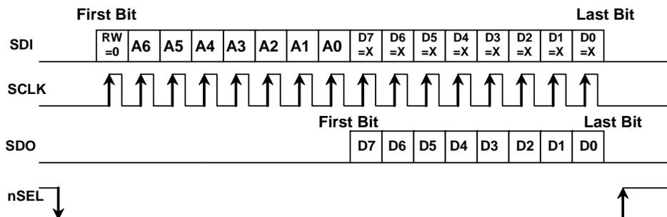
**Figure 3. SPI Timing—READ Mode**
