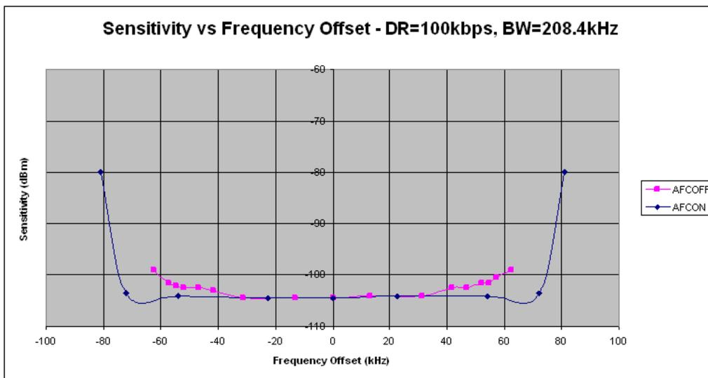
Figure 8. Sensitivity at 1% PER vs. Carrier Frequency Offset
