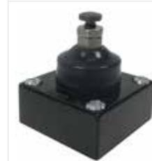
**BXV - Adjustable top pin plunger:** A copper alloy adjustable plunger provides easy application and saves on installation time. The operating points of the switch can be adjusted from 52,8 mm to 59,3 mm [2.085 in to 2.335 in]. Seals are the same as the pin plunger.
