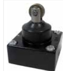
**BXD/BX2D - Top roller plunger:** A copper alloy roller plunger is adjustable to 90° angles to accept cam or slide operation from any of two directions. Boot seal on the plunger.
