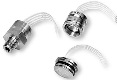
Honeywell's stainless steel 19C, 19U, and 19 Vacuum Gage Series sensors were developed for pressure applications that involve measurement of hostile media in harsh environments compatible with 316 stainless steel. The special Vacuum Gage Series sensors are specifically designed for applications that can be exposed to vacuum.
