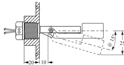
N.O. function, i.e. the contact closes when the liquid level rises.
