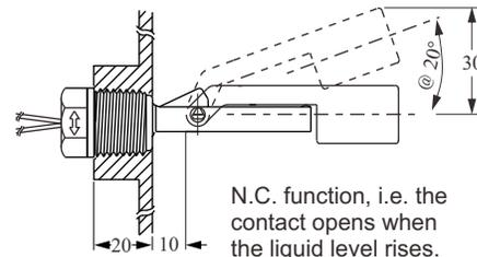
N.C. function, i.e. the contact opens when the liquid level rises.
