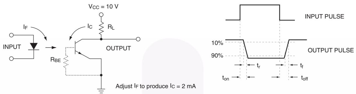
Figure 8. Switching Time Test Circuit and Waveforms
