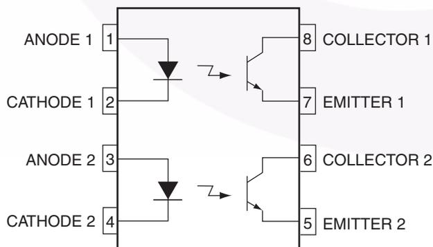
Figure 1. Schematic
