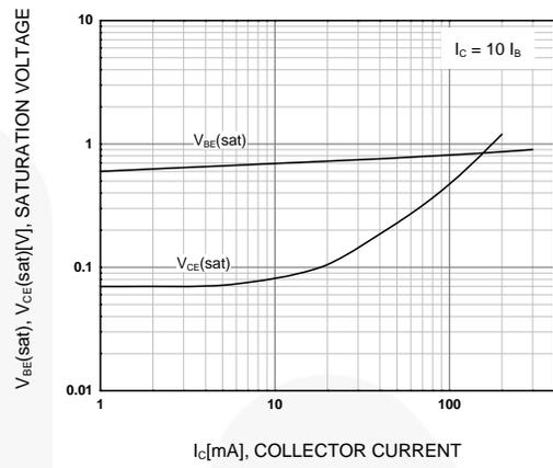
Figure 2. Collector-Emitter Saturation Voltage and Base-Emitter Saturation Voltage
