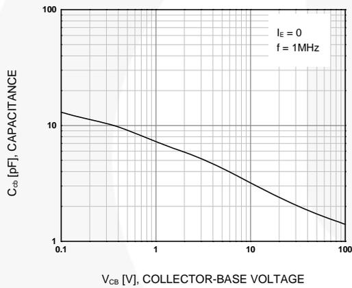
Figure 3. Collector-Base Capacitance
