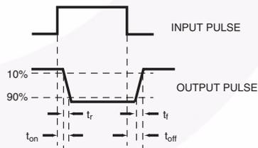
**Figure 11. Switching Time Test Circuit and Waveforms**
