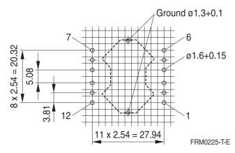
Hole arrangement View in mounting direction (Note half pitch!)
