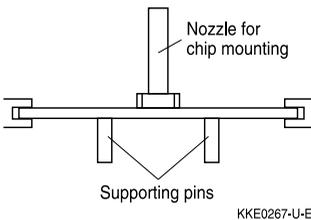
It is recommended that the PC board should be held by means of some adequate supporting pins such as shown left to prevent the SMDs from being damaged or cracked.
