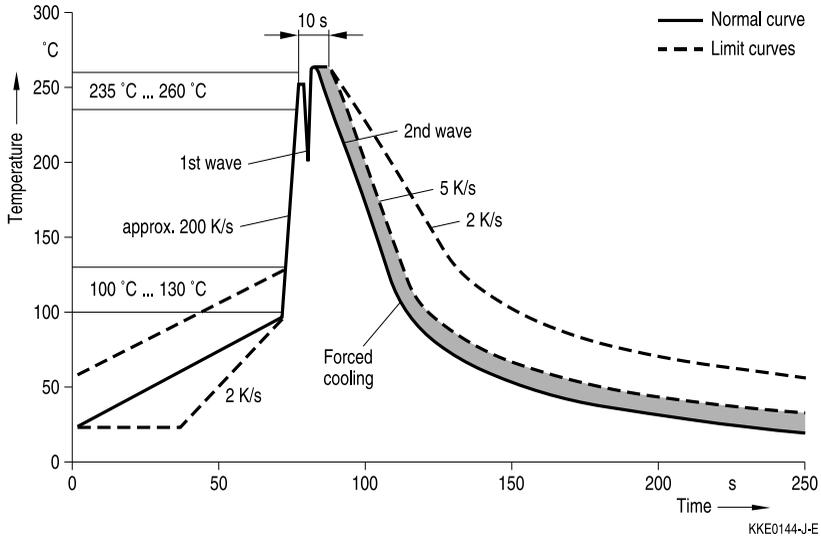
**Solder joint profiles for silver/nickel/tin terminations**
