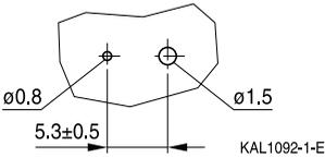
Suggestion for PCB hole diameter, wire  $\varnothing 0.8$  mm
