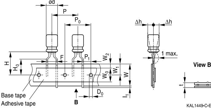
**Lead spacing 5.0 mm (∅ d = 10 ... 12.5 mm)**
