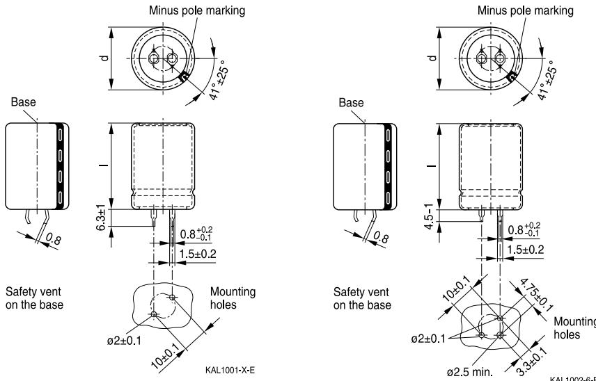
Snap-in terminals, length  $6.3 \pm 1$  mm. Also available in a shorter version with a length of  $4.5 - 1$  mm. PET insulation is marked with label "PET" on the sleeve.
